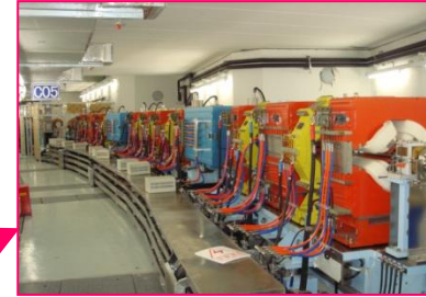
3.5GeV storage ring, with length 432m
